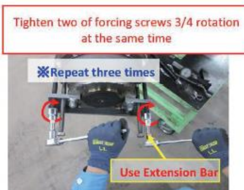
Figure 10 Tighten forcing
