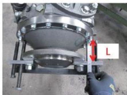
Figure 9 Measure the distance between the front axle cover and Jig.
