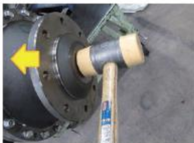
Figure 13 The axle that found out OK, put the front axle shaft into the case by hitting the front axle with a plastic hammer
