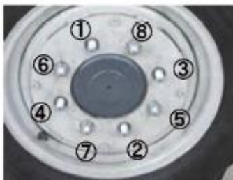
Figure15 Tighten wheel bolts and nuts.
