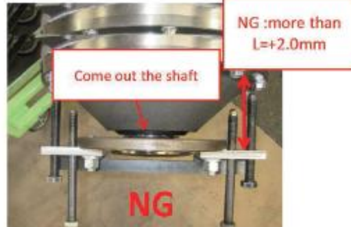
Figure12 NG Circlip missing
